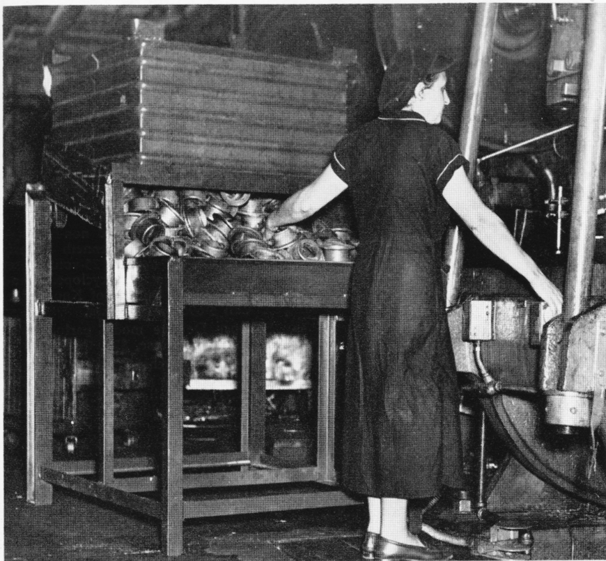
Mary Vellucci demonstrates how conveniently she can take work from the new Work-O-Matic drop-bottom steel box which is set up on a steel stand. This new equipment eliminates the use of work pans which had to be disposed of, by the operator, as each was emptied.
